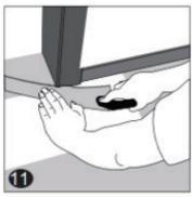
1. After thoroughly cleaning the subfloor, you should begin laying from left to right. Position the first plank so that grooved edge is facing you. Place the floorboard 1/4" (6mm) from the left wall. Use spacers between the wall and the floorboard.
